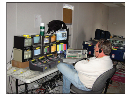
Figure 7.54 Here is a super slow-motion (known as super "slo-mo" in industry slang) instant replay operator during a break in the action. This replay is "super" because it records at 90 frames a second instead of the 30 frames normal for NTSC. This allows for much smoother motion from frame to frame upon playback. This "table-top" remote was in addition to the production truck's usual complement of equipment and was therefore set up in an office trailer in the compound and interconnected into the truck as an integral part of the system.
